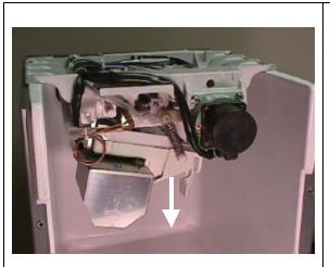
The actuator motor turns counter clock wise to rotate the cam arms and lower the water pan away from the evaporator. When the water plate is completely down the switch lever moves the actuator toggle switch to the left. The board energizes the inlet water valve and condenser fan motor and de-energizes the hot gas valve.
